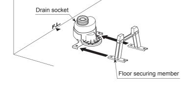
(3) Drill the pilot holes (ø11 mm, 55 mm deep) at the positions marked in step (2). Completely remove chips, and then insert the floor securing AY bolts. Push the edge of the rubber tube into the the hole, pull the bolt in the tube hard to expand the rubber tube to form complete contact with the hole, and then unscrew the bolt to remove it.
