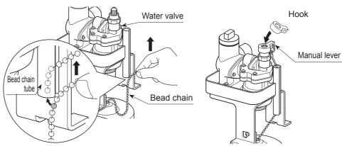
Insert the thin section between beads near the manual lever through the slit into the bead chain tube, and pull the chain up. The entire bead chain is inserted in the tube.
