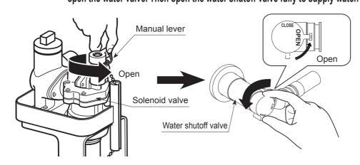
2. Open and close the manual lever several times to check that there is no water leaking at connecting sections.
