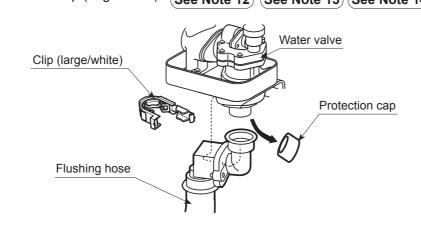
(3) After the clip (large/white) has been attached, turn the clip to check that the clip is engaged with the groove correctly.
