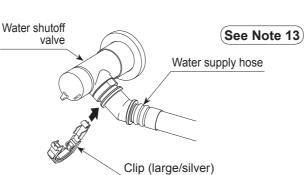
(3) After the clip (large/silver) has been attached, turn the clip to check that the clip is engaged with the groove correctly.
