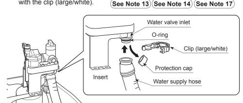
(3) After the clip (large/white) has been attached, turn the clip to check
