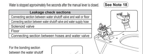
valve and wall, lift the ring shaped cover and the water supply pipe cover to check that there is no water leakage.
